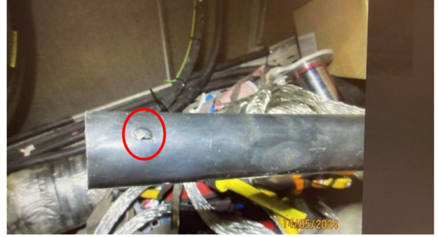
Fig. 13. Large localized hump at the semiconductor layer of the cable
