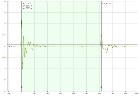
Fig. 2. Direct and reflected pulse when the remote end is open
