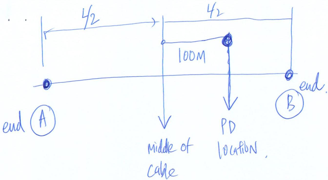
④ cable length can be measured by separate TDR and say it is 450M.
