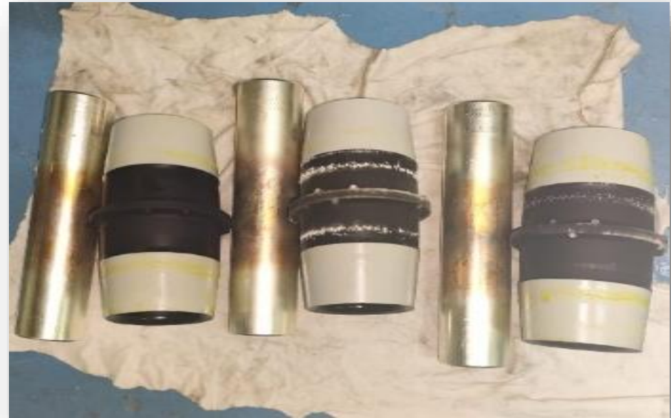
Visible discharge busbar of GIS
